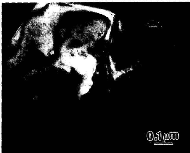
Fig. 6. TEM micrograph (dark field image) showing the intragranular particle-induced dislocations developing into a microcrack (sample L_6 ).
