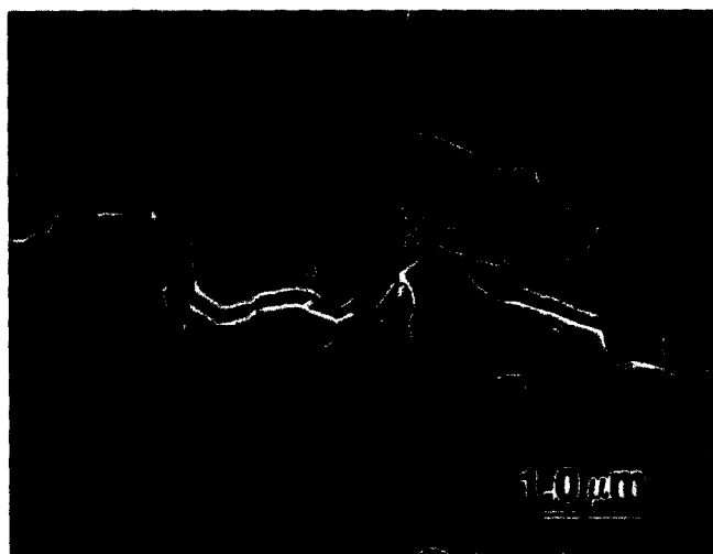
Fig. 4. SEM image showing a significant crack deflection was caused by an \sim 1\text{-}\mu\text{m} -long intergranular SiC particle (sample L 12 ).
